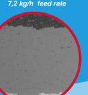
SG DV1196 - Al<sub>2</sub>O<sub>3</sub> 2% porosity - 65% DE 2,9 kg/h deposition rate 4,5 kg/h feed rate
